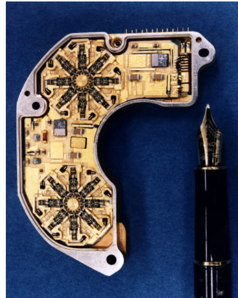
Figure 8. Combiner Side View of W-Band Transmitter Assembly
