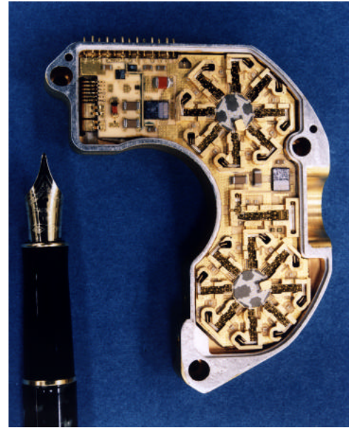
Figure 7. Divider Side View of W-Band Transmitter Assembly
